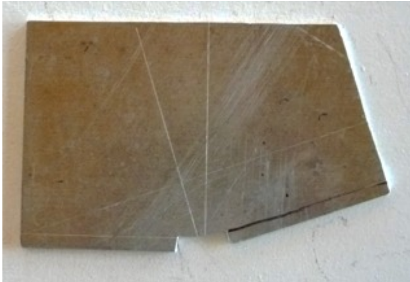
Figure 3 Jig for determining Genoa luff intersection with front face of the mast. The Genoa halyard is held parallel to the edge (i.e. at 18.4^{\circ} along the red arrow) and no part of the Genoa sail shall be in front of the line on the jig which is at 5 mm from the edge.
