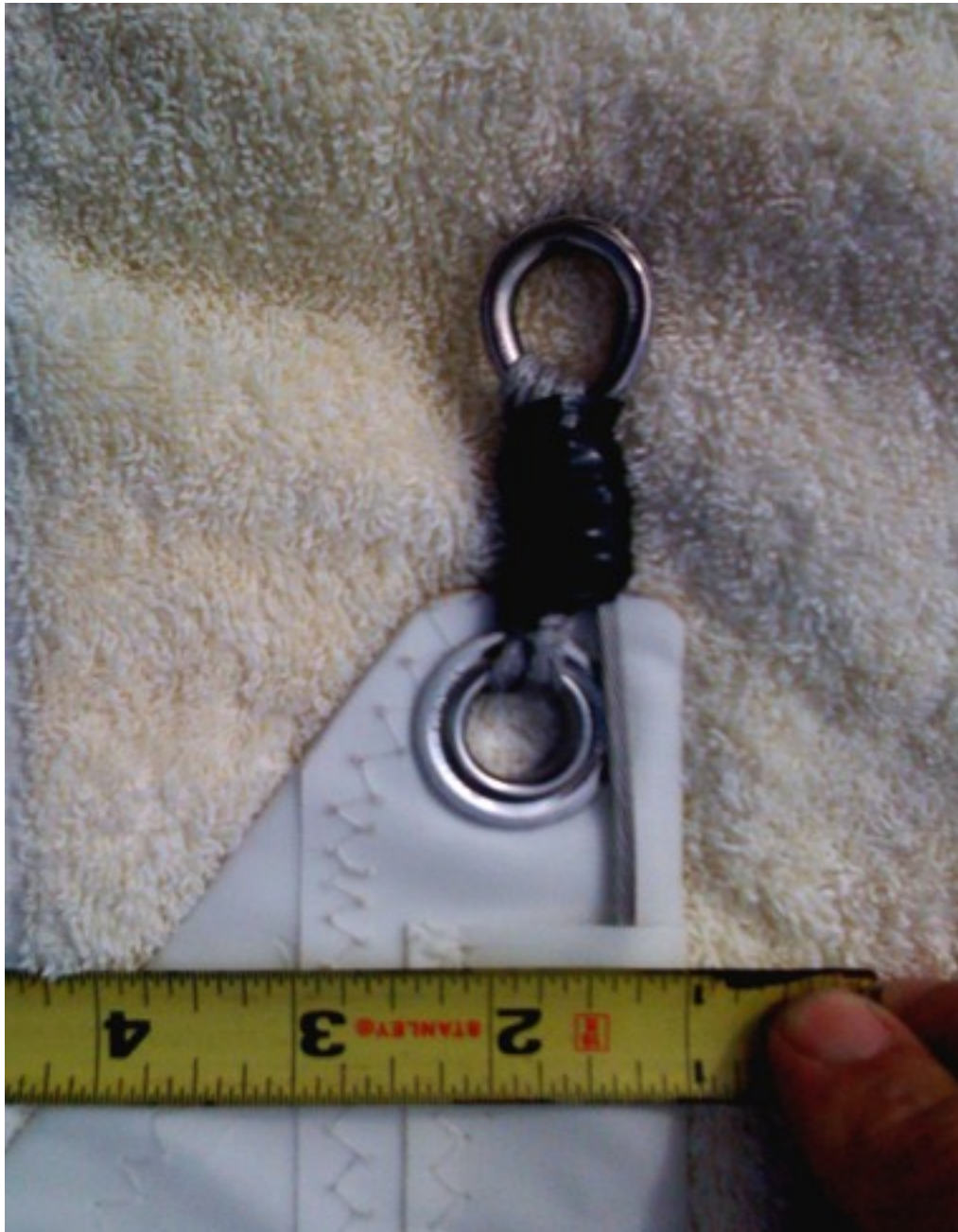
Figure 4 The head of a North FD Genoa showing that this sail head point extends 8 mm in front of the leading edge of the luff wire.
