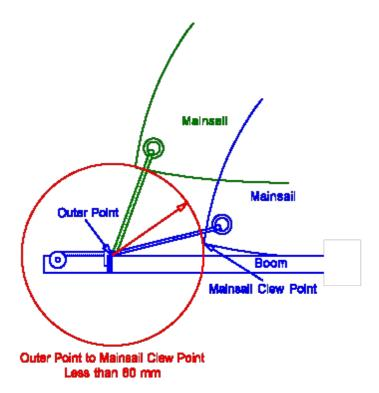
This rule then requires a physical stop, i.e. the strap (as is the case for mainsails in a foot grove) which prevents the clew of the sail being rigged beyond the outer point, but also restricts the mainsail clew from flying free more than 60 mm from the outer point on the boom.
